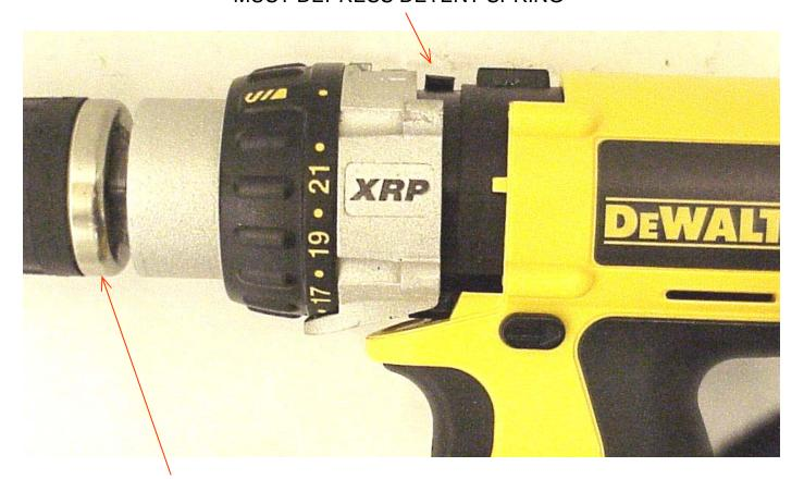
WHILE APPLYING LIGHT AMOUNT OF PRESSURE ROTATE CHUCK TO ENGAGE SPINDLE IN TRANSMISSION
